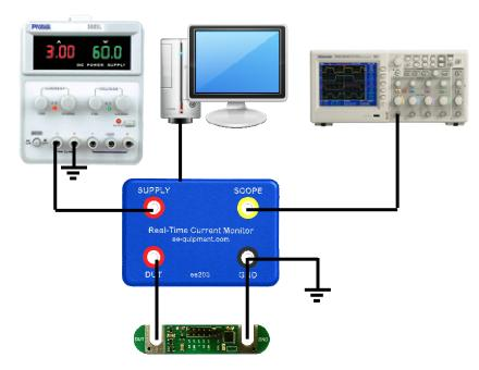
Connect the PC, oscilloscope, Current Monitor, and DUT as shown.
