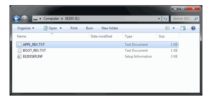
To verify that a programming operation has been successful, detach and reattach the USB cable after programming to allow the PC to re-enumerate the ee203. Then check the appropriate text file to confirm that the desired firmware revision has loaded.
